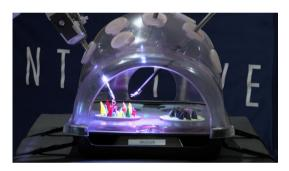
Figure 2 Plastic model for exercising port placement, docking, undocking and simple dexterity.
