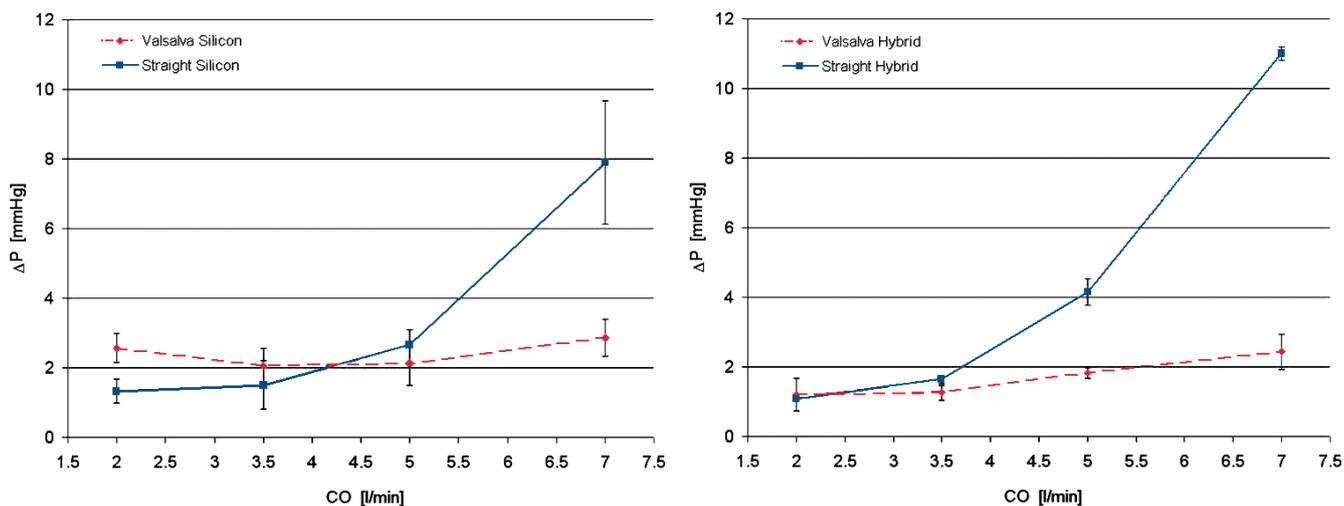
**Figure 3** Pressure drop across the valve in both roots, with and without sinuses, either made out of silicon (standard compliance) or made out of Dacron (minimized compliance). Note that independent of root compliance, the absence of sinuses increased the pressure drop across the valve. (Reprinted from J Thorac Cardiovasc Surg, Elsevier, with permission)
