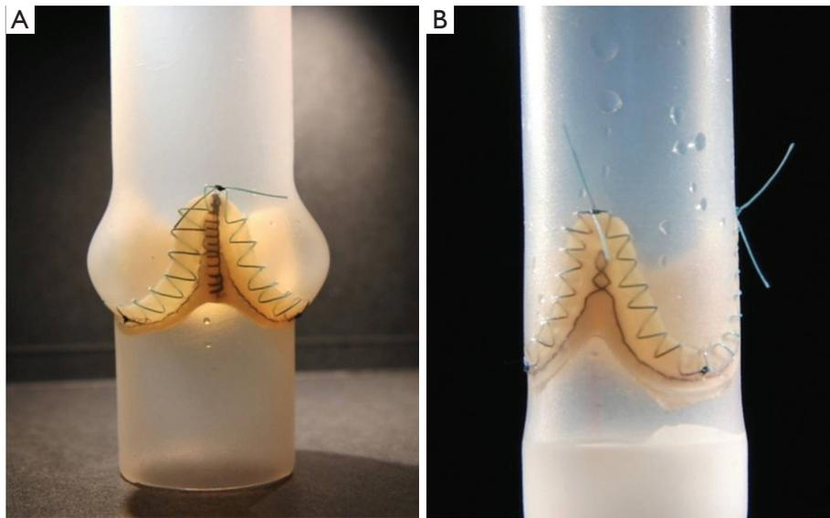
**Figure 1** The two root silicon models with the same compliance, but either with or without sinuses. A stentless valve was sutured inside following the remodeling techniques. (Reprinted from J Thorac Cardiovasc Surg, Elsevier, with permission)
