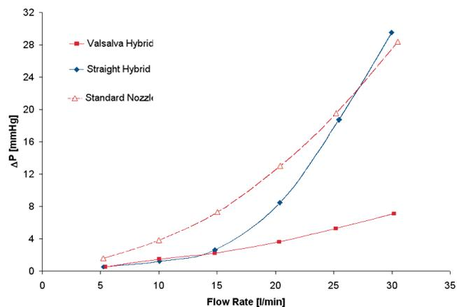
**Figure 4** Pressure drop across the valve in both Dacron roots, with and without sinuses, compared with a standard nozzle. Note that when steady flow becomes turbulent (i.e., around 15 L/min) the presence of sinuses helps to maintain a low pressure drop across the valve
