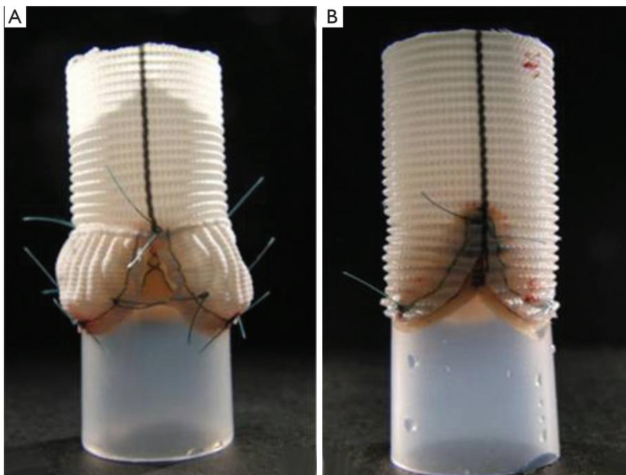
**Figure 2** The silicon models where the upper part was substituted with a straight or a Valsalva Dacron graft to minimize the role played by root compliance. (Reprinted from J Thorac Cardiovasc Surg, Elsevier, with permission)
