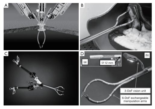
**Figure 3** Examples of Single Port Access Surgery Equipment. (A) da Vinci Single Site Surgical Robot (15); (B) Titan Surgical Robot (16); (C) Spider surgical system (17) and (D) SJTU unfoldable robotic system (18).
