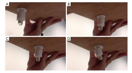
**Figure 2** (A) Wireless steerable endoscope (WSE) prototype: the WSE is held against gravity by a magnet under a wooden plank mimicking attachment to the internal wall of a body cavity and is able to (B) slide; (C) axially rotate; (D) providing multiple viewing directions.
