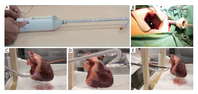
Figure 1 The cardioscope during testing: (A) the cardioscope prototype; (B) retroflexion of the cardioscope in an animal model of thoracic surgery; (C) the cardioscope operating at a short bending section; (D) the cardioscope operating at a longer bending section; (E) the cardioscope guiding other operating tools through a simulated uniportal approach.
