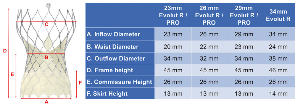
Figure 4 Repositionable self-expanding valves with and without an external pericardial wrap: features and dimensions. Various dimensions of the Evolut-R and Evolut-PRO CoreValve (Medtronic, Galway, Ireland) are listed for comparison. Reprinted from ref (25), with permission from Elsevier.
