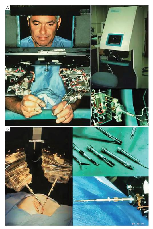
**Figure 6** The first surgical robot prototype. (A) Green telepresence surgeon's workstation with hand controls—Stanford Research Institute 1994. (B) Exchangeable end-effector surgical instruments. The figure is reproduced with permission from the *Journal of Laparoscopic Surgery and Society of Laparoscopic and Robotic Surgeon*.
