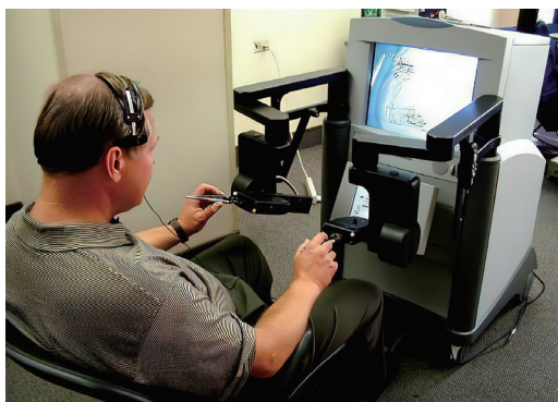
Figure 8 The ZEUS operating console with voice activated endoscope position control.
