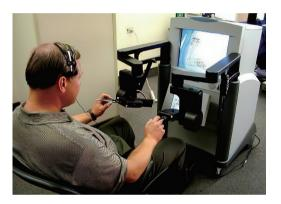
Figure 8 The ZEUS operating console with voice activated endoscope position control.
