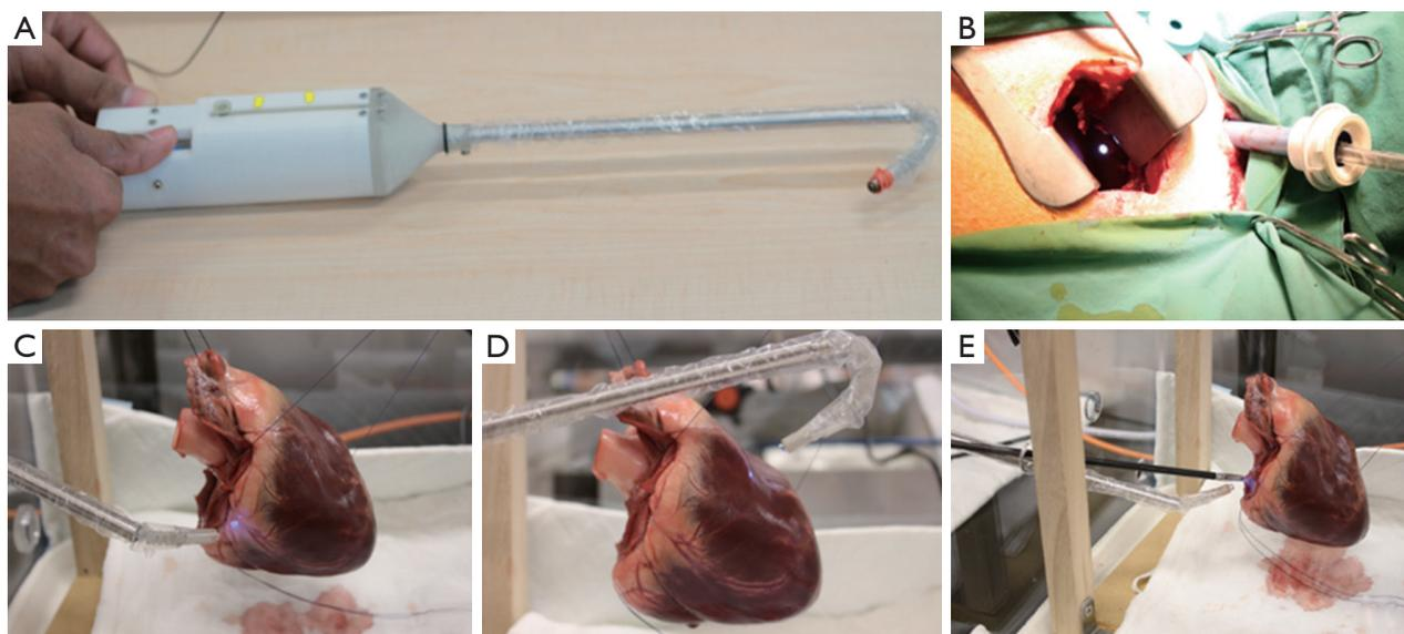
**Figure 1** The cardioscope during testing: (A) the cardioscope prototype; (B) retroflexion of the cardioscope in an animal model of thoracic surgery; (C) the cardioscope operating at a short bending section; (D) the cardioscope operating at a longer bending section; (E) the cardioscope guiding other operating tools through a simulated uniportal approach.
