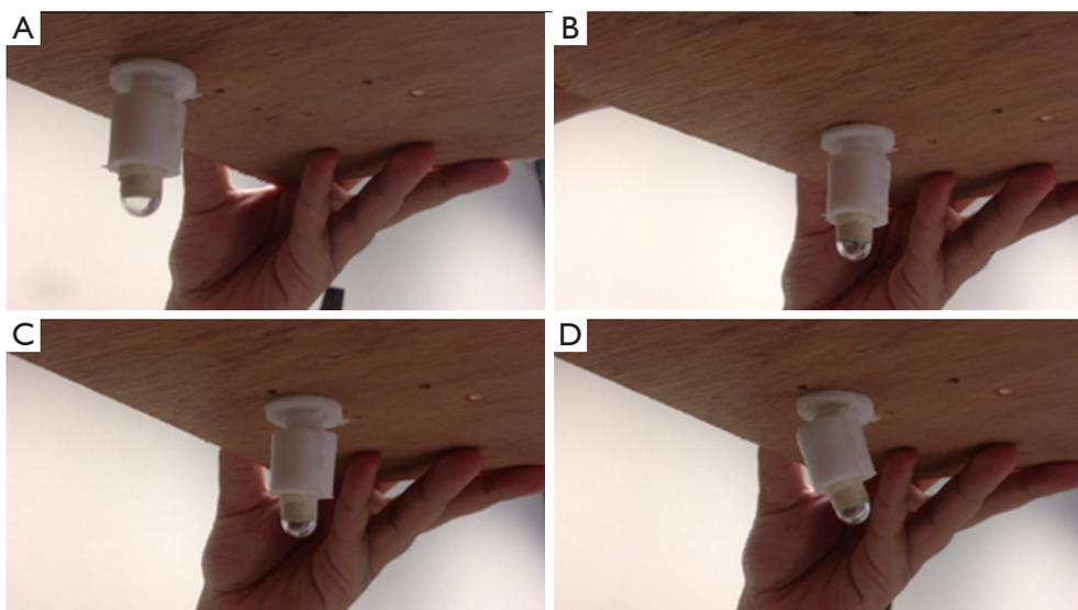
**Figure 2** (A) Wireless steerable endoscope (WSE) prototype: the WSE is held against gravity by a magnet under a wooden plank mimicking attachment to the internal wall of a body cavity and is able to (B) slide; (C) axially rotate; (D) providing multiple viewing directions.
